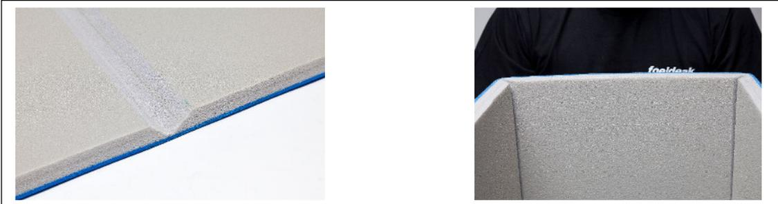
Ideally, this V groove is cut by means of a buzz saw in two steps with the saw blade inclined to 45 °. We recommend using a fine saw blade and a guide rail. (Given exact dimensions, the mat elements can be prepared accordingly in our production.)
